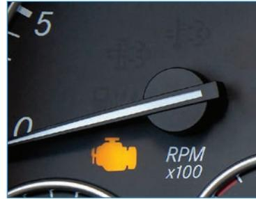
If you see the MIL and check engine light on at the same time, you may experience an engine derate — where the computer reduces engine power to protect the engine and limits road speed. This situation needs to be reported to your support team as soon as possible. Ensure you're in a safe place (preferably at a repair shop) before you shut off your engine in this situation as depending on the problem you may be limited to a speed of 8 km/h upon restart until the issue is repaired.
