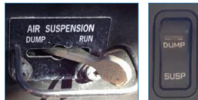
Wait for the airbags to inflate before driving away. Driving with the airbags deflated will cause damage to the tractor driveline components such as the driveshaft, constant velocity (CV) joints, the differential, axle shafts and universal joints (U joints).
