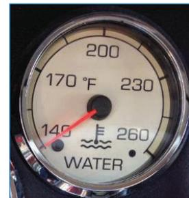
Overheating can happen when there are low coolant levels, a sudden loss of coolant or severe operating conditions such as climbing a steep grade.
