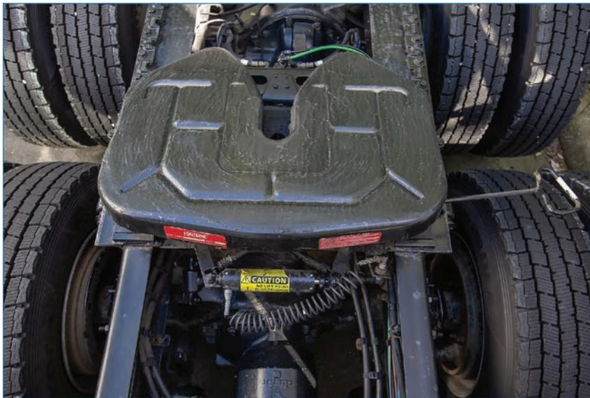
**Fifth wheel slide lock** — Used to slide the fifth wheel to various positions in order to adjust weight distribution between the steering axle and the drive axles, as well as to accommodate a trailer with a deep kingpin setting, for example.
