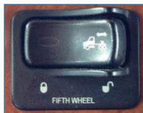
Generally once the fifth wheel has been set you don't have to move it again. Never operate the vehicle with the switch in the unlock position. Always ensure the switch is in the lock position and the pins are locked in place before driving the vehicle. Otherwise, the trailer could come unhitched from the tractor.
