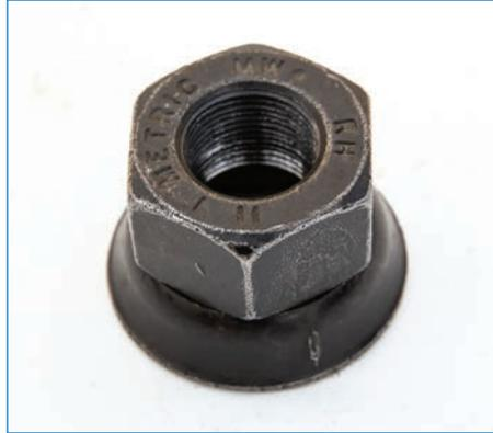
**Note:** All wheel nuts, for all types of wheels, must be checked that they're tight and are torqued by a qualified installer. After installation it's required to get wheels retorqued usually within 150 km. Make sure you pay extra attention to any recently installed wheels during your vehicle inspections to ensure they're staying tight.
