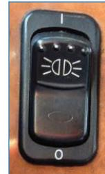
**Marker interrupter/ID and clearance lights flash** — Generally used at night to thank other drivers who assisted you in passing them. It can be a switch on the dash or a button on the end of the headlight dimmer lever located on the steering column. Some trucks have this button on the steering wheel.
