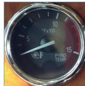
If excessive exhaust temperatures occur, give the engine a chance to cool by gearing down to raise the engine RPM. If the other gauges are also outside of their normal ranges, the problem might be more serious. Stop and find the cause of the problem. Refer to your owner's manual for normal operating temperatures.
