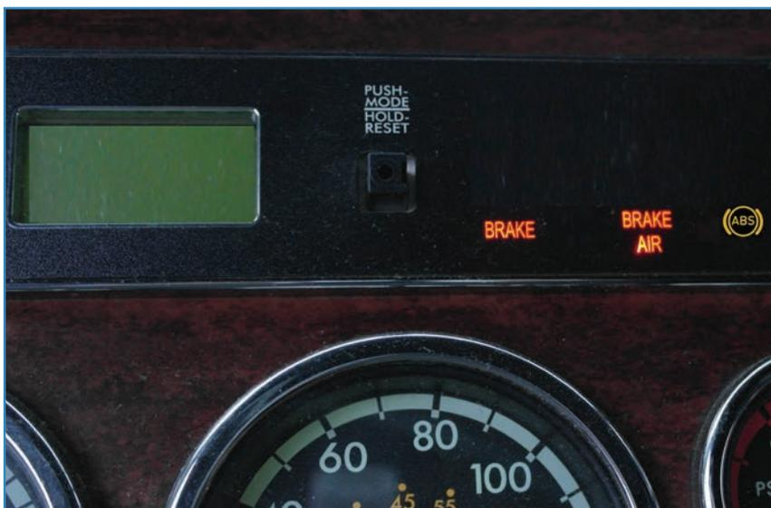
Vehicles are equipped with a dash-mounted failure warning light that monitors the ABS. When the ignition switch is first turned on, the ABS performs a self-checking sequence. Depending on the system, the warning light may turn on, flash briefly, then stay lit until vehicle speed reaches seven kilometres an hour to 11 km/h or light briefly then turn off.
