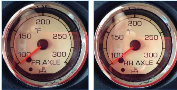
It's normal for the front axle to read higher than the rear axle. High temperature readings indicate you should check the axle lubrication.
