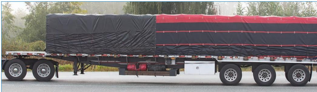
Monitor the tarp for problems while driving. A flapping tarp is caused when a tarp has been improperly secured or a tarp grommet has ripped out. This will damage the tarp, expose the cargo and prevent you from seeing the rear end of the load. You must also be cautious of wind getting under the tarp and causing a ballooning effect.
