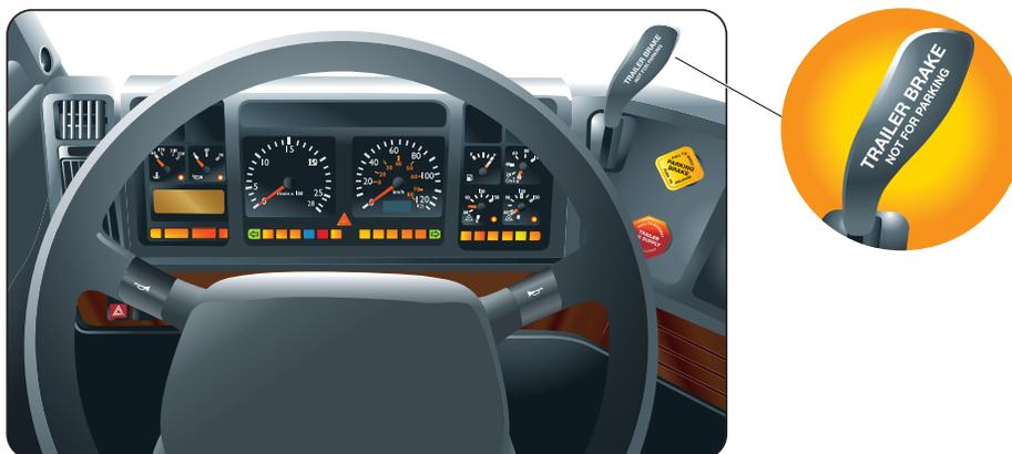
For this you use the hand valve. When the trailer air brake system is fully connected to the tractor, the hand valve allows you to apply the trailer service brakes independently of the tractor.
