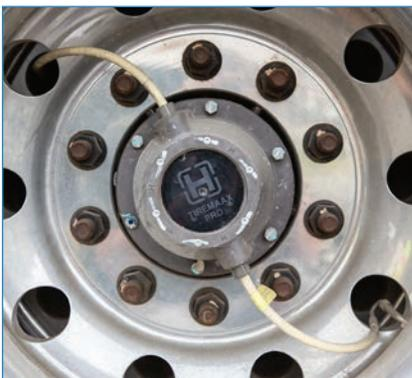
**Rims** — Tires are mounted on rims or wheels that are then installed on your truck or trailer. A one-piece rim is used for tubeless tires (radials) which are most common today.
