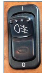
**Work light/utility lights** — Most truck tractors come equipped with lights mounted to the side of the cab or bunk. Use these lights at night when backing up, coupling and uncoupling, chaining up or doing circle check inspections. This switch will either be located on the dash or a toggle switch will be installed on the inside of the cab wall behind the driver's seat.
