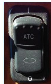
When on, a wheel spin control warning light will illuminate when drive wheel spin is detected and power will be reduced until the wheel stops spinning.
