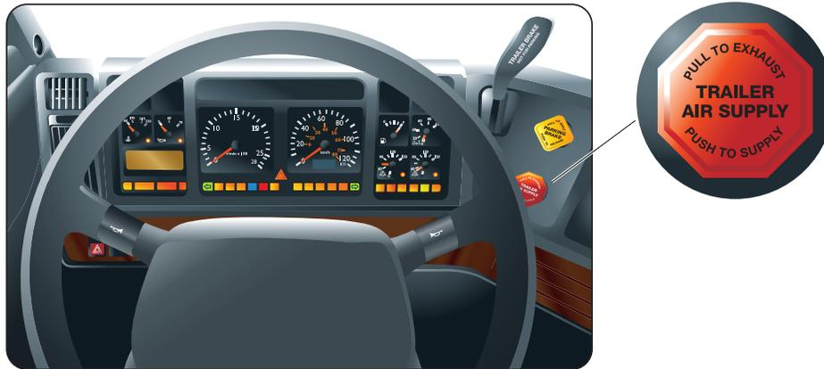
For this, you use the dash-mounted trailer air supply valve, which senses air pressure in the supply line that carries air to the trailer system. Most trailer air supply valves are an octagon-shaped red button.
