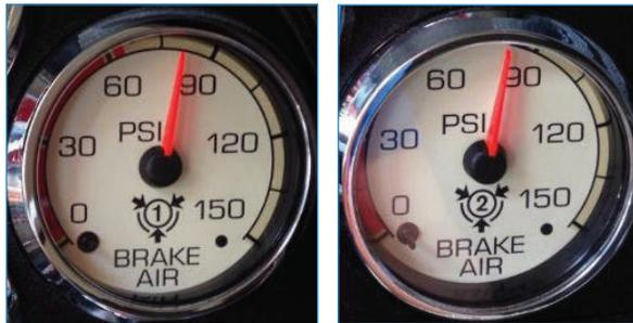
Other option: Single dual air pressure gauge with two different coloured needles indicating primary and secondary air system.
