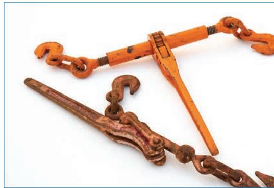
The requirements for chaining down a load (for example, the number of tie downs required on a flatbed) are covered in Motor Vehicle Act Regulations Division 35 — Cargo Securement. The weakest link, whether it's the chain, hook or binder, will determine the allowable SWLL.
