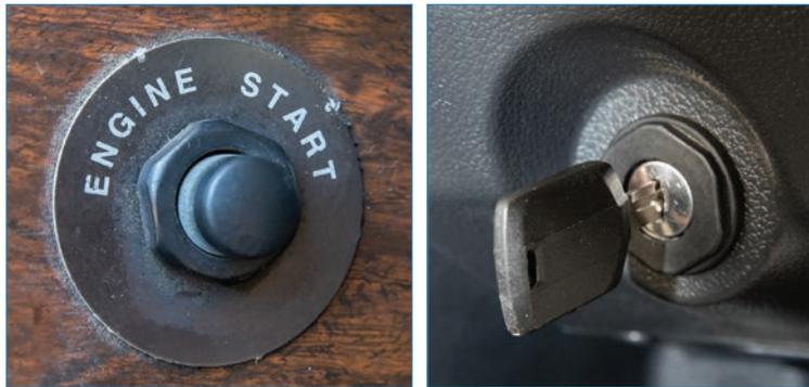
Some older trucks will have a separate ignition switch and then a push button to start the engine. Most late model trucks have the same style ignition/start/accessory key switch as most cars and light trucks today.
