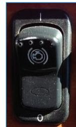
Ensure you have adequate traction between the drive tires and the road surface before activating the engine brake or you could create a dangerous jackknife situation. There are four types of auxiliary brakes (engine brake, exhaust brake, hydraulic retarder and electric retarder). More information can be found in the air brakes unit.
