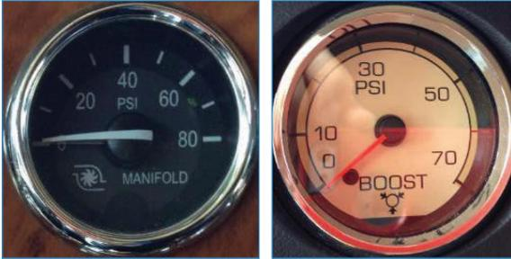
The amount of p.s.i indicated on the gauge will vary depending on the load placed on the engine. If the pressure goes down when the engine is under a load, there may be something wrong with the engine and it should be checked by a mechanic.
