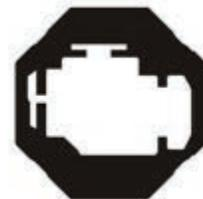
**Wait to start engine** — Illuminates yellow when the intake air heater (grid heater) needs to warm the intake air, or glow plugs need to warm the cylinder, before starting the engine.
