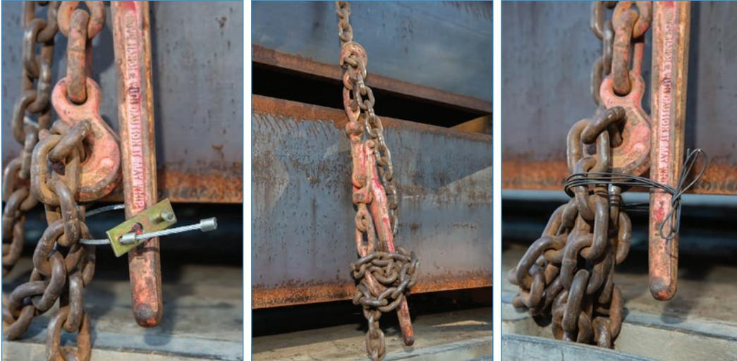
All tie downs and other parts of a cargo securement system must be located inside any rub rails whenever practical. Edge protection must also be used whenever a tie down would be subject to wear or cutting at the point where it touches an article of cargo. The edge protection must resist wear, cutting and crushing.
