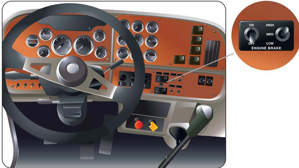
To activate the retarder, there is an on/off switch and a switch to vary the amount of holdback. If the switch is turned on and you release the pressure on the throttle pedal and clutch, the retarding device will activate.
