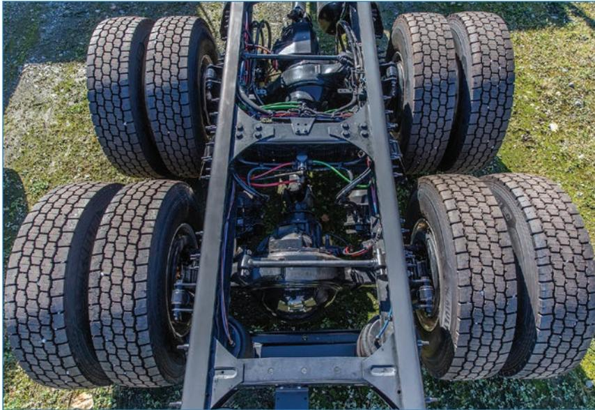
**Tri-drives** — Three axles systems or tri-drives distribute power to three live axles to provide additional traction.
