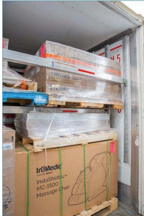
5. **Load locking bars** — used vertically or horizontally, these bars have rubber feet that are placed against the vehicle walls or ceiling and floor. The bars are placed snugly against the cargo and then tightened with a jacking device until they're tightly wedged in place against the cargo. Jack bars no longer have a weight rating for securing cargo and need to be supplemented with other securement devices as required to meet the regulations.
