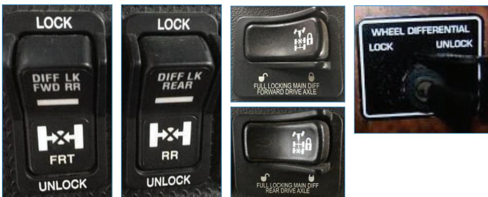
Move the switch to the lock position to lock the wheels together.
