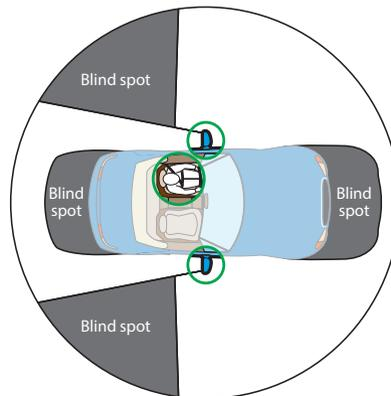
**Blind spot detectors, cameras** — Some vehicles are equipped with blind spot detectors and/or back-up cameras. While these can help you to detect hazards in blind spots or behind the vehicle, they do not replace the need to turn your head to do a shoulder check or look behind.
