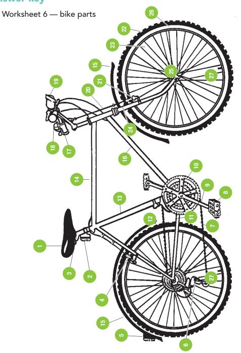
1 Seat 2 Rear light 3 Seat stay 4 Rear calliper brake 5 Red rear reflector 6 Rear derailleur 7 Chain 8 Pedal 9 Crank arm 10 Chain ring 11 Chain stay 12 Front derailleur 13 Seat tube 14 Top tube 15 Fenders 16 Down tube 17 Handlebar grip 18 Bell 19 Front light 20 Brake cable 21 Front calliper brake 22 Tire 23 Spokes 24 Fork 25 Hub 26 Rim 27 Tire valves
