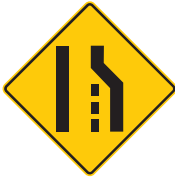
Right lane ends ahead
