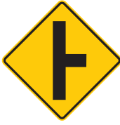
Hidden side road ahead
