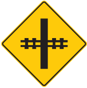
Railway crossing ahead — be prepared to stop
