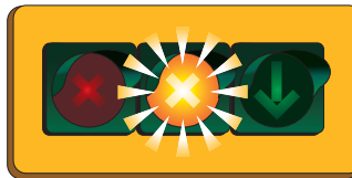
Move out of this lane and into a lane with a green arrow. If the lane control signals over all of the lanes are flashing yellow, slow down and proceed with caution
